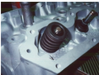
Bead Blasted Head with new Valves, Springs, Retainers, etc.
